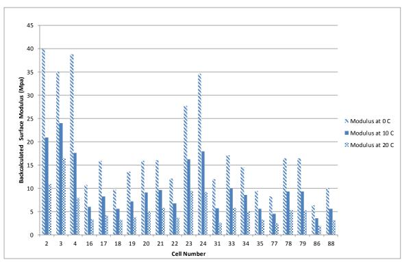
Figure 22: Change in backcalculated moduli at different temperatures
