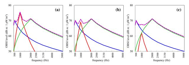
Figure 2. Fitting constituent spectra to measured noise. The mid-frequency spectrum (red) is adjusted higher or lower such that the sum of the three constituent spectra (black dotted) matches the measured spectrum (magenta) for each of the three pavements (a), (b) and (c)
