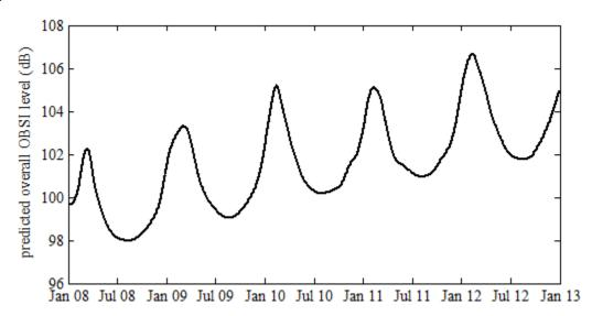
Figure 30: Predicted change in overall OBSI level of a typical pavement over time (RoboTex).
