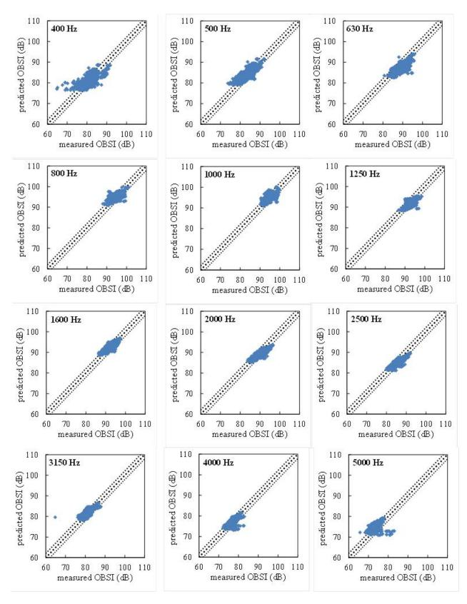
Figure 45. Measured and predicted one-third octave band levels, leading edge, RoboTex model.
