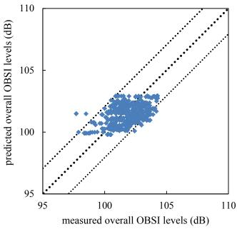
Figure 37. Measured and predicted overall OBSI levels, leading edge, CTM data. Dotted line: 1:1.
