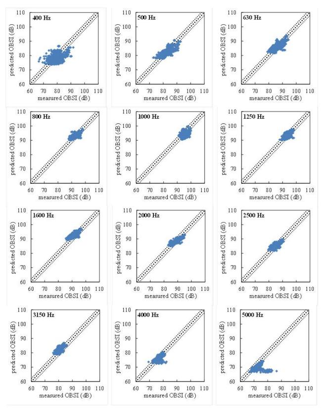
Figure 46. Measured and predicted one-third octave band levels, trailing edge, RoboTex model.
