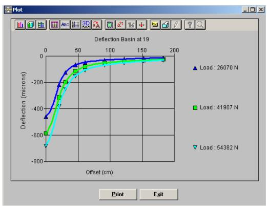
Figure B 3: Plot of deflections basins measured for Cell 19 at different loads.
