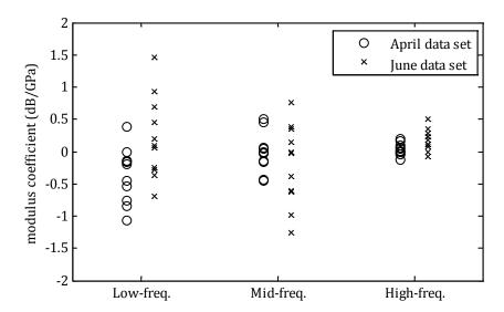
$Figure\ C\ 9:\ Best-fit\ modulus\ coefficients\ for\ two-parameter\ temperature-modulus\ model.$
