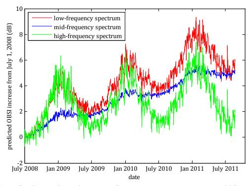
Figure 20: Predicted increase in constituent spectra from two-parameter age-temperature model from July 1, 2008.
