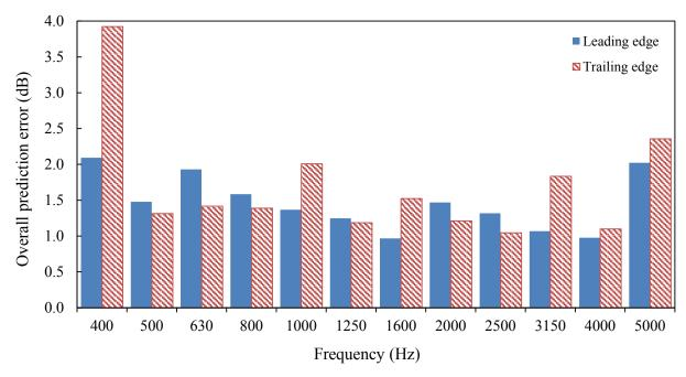
Figure 47. RoboTex Model accuracy by one-third octave bands.
