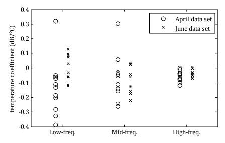
Figure C 8: Best-fit pavement temperature coefficients for two-parameter temperature-modulus model (trailing edge).
