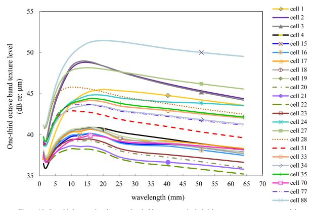
Figure 10: One-third octave band texture levels 22 pavements included in one-parameter texture model.
