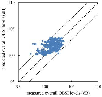
Figure 38: Measured and predicted overall OBSI levels, trailing edge, CTM data. Dotted line: 1:1.
