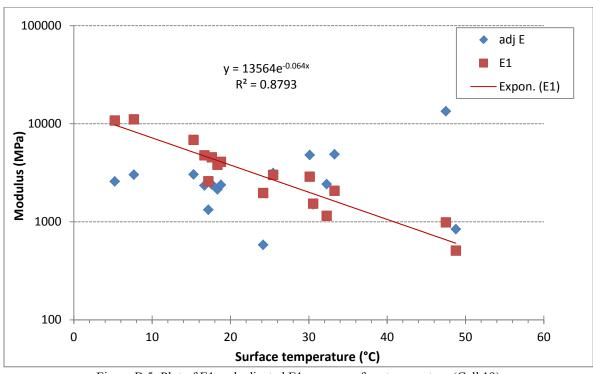
Figure B 5: Plot of E1 and adjusted E1 versus surface temperature (Cell 19).
