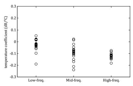
Figure 18: Best-fit temperature coefficients for two-parameter age-temperature model.
