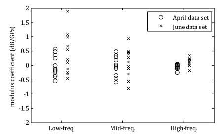
Figure 24: Best-fit modulus coefficients for two-parameter temperature-modulus model.
