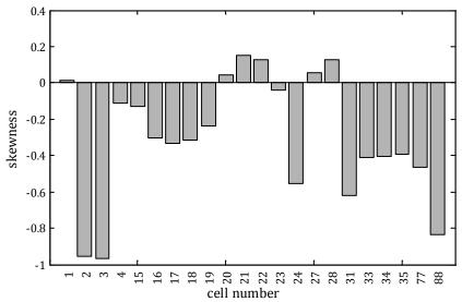
Figure 14: Skewness for 22 pavements included in one-parameter skewness model.
