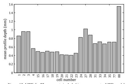
Figure 13: MPD for 22 pavements included in one-parameter MPD model.
