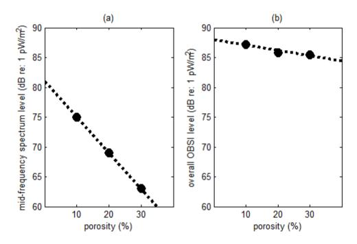
Figure 3. Comparison of the level of the mid-frequency component results from (a) mechanism decomposition approach and (b) overall level approach. The mechanism decomposition approach leads to better insights about the effects of porosity on the three pavements.
