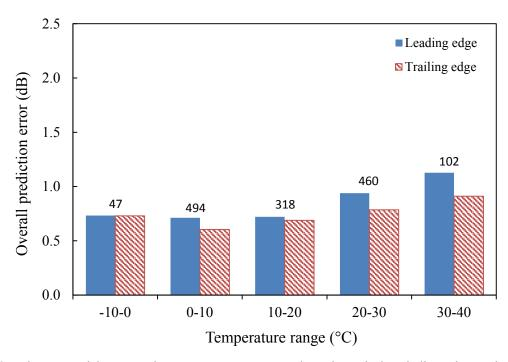
Figure 43. RoboTex Model accuracy by temperature range. Numbers above the bars indicate the number of OBSI measurements included for that temperature range in the model.
