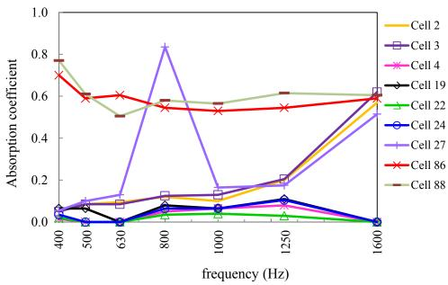
Figure 15: Absorption spectra for nine pavements included in one-parameter absorption model.
