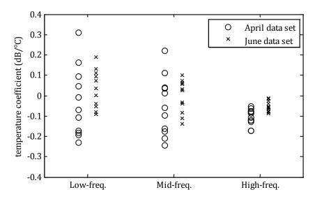
Figure 23: Best-fit pavement temperature coefficients for two-parameter temperature-modulus model.
