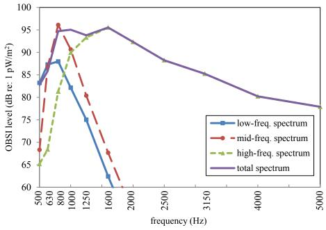
Figure 6: Combination of constituent spectra to form total OBSI spectrum.
