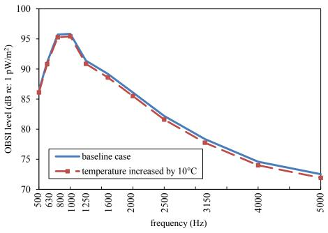
Figure 34. Effect of increased temperature, taking change in modulus into account (CTM).
