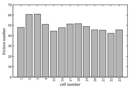
Figure 17: Friction numbers for 13 pavements used in one-parameter friction model.
