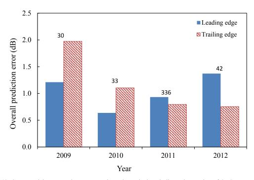
Figure 42. CTM Model accuracy by year. Numbers above the bars indicate the number of OBSI measurements included for that year in the model.
