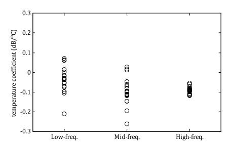
Figure C 6: Best-fit temperature coefficients for two-parameter age-temperature model (trailing edge).
