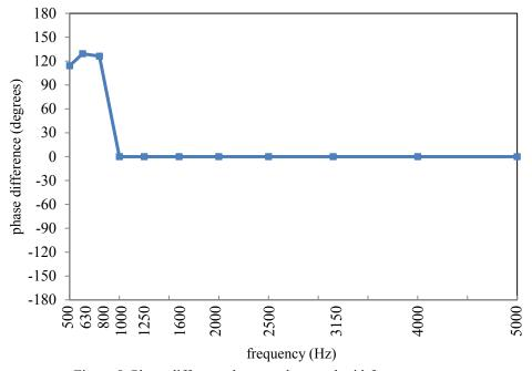
Figure 5: Phase difference between low- and mid-frequency sources.
