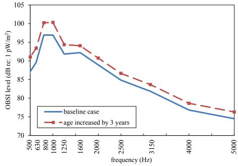
Figure 27: Effect of increased pavement age (RoboTex).
