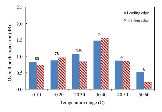
Figure 44. CTM Model accuracy by temperature range. Numbers above the bars indicate the number of OBSI measurements included for that temperature range in the model.
