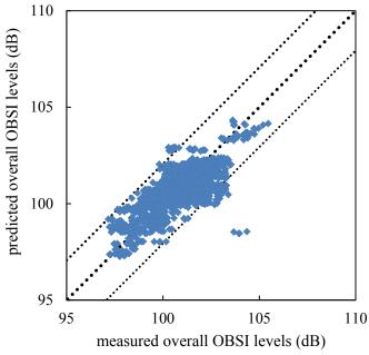
Figure 36: Measured and predicted overall OBSI levels, trailing edge, RoboTex data. Dotted line: 1:1.
