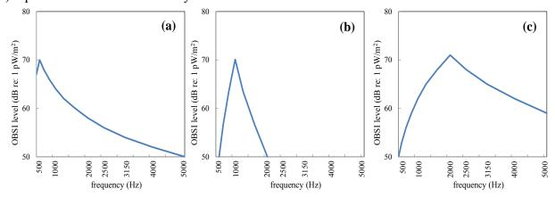
Figure 1. Example constituent spectra. (a) low-frequency spectrum, affected by macrotexture; (b) mid-frequency spectrum, affected by prosity; (c) high-frequency spectrum, affected by friction.
