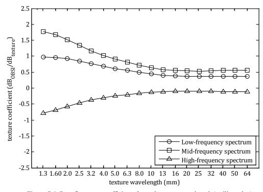
Figure C 4: Best-fit texture coefficients for each texture wavelength (trailing edge).
