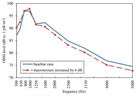
Figure 25: Effect of increased macrotexture (RoboTex).
