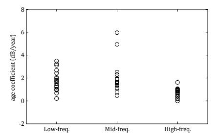
Figure 19: Best-fit pavement age coefficients for two-parameter age-temperature model.
