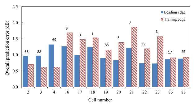
Figure 40. CTM Model accuracy by cell. Numbers above the bars indicate the number of OBSI measurements included for that cell in the model.
