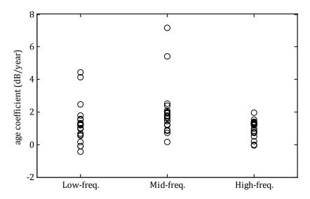
Figure C 7: Best-fit pavement age coefficients for two-parameter age-temperature model (trailing edge).
