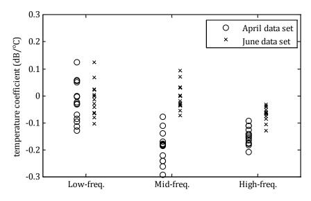
Figure C 2: Constituent spectra temperature coefficients using air temperature (trailing edge).
