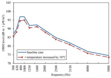
Figure 29: Effect of increased temperature, taking change in modulus into account (RoboTex).
