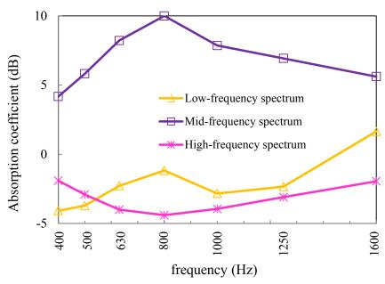
Figure 16: Best-fit coefficients for each absorption frequency.
