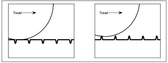
Figure A 1: Positive and negative texture for two pavements with identical texture spectra. Left: Negative texture. Right: Positive texture.
