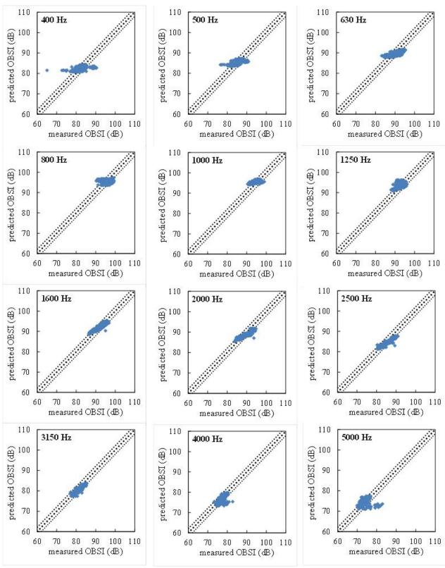
Figure 48. Measured and predicted one-third octave band levels, leading edge, CTM model.
