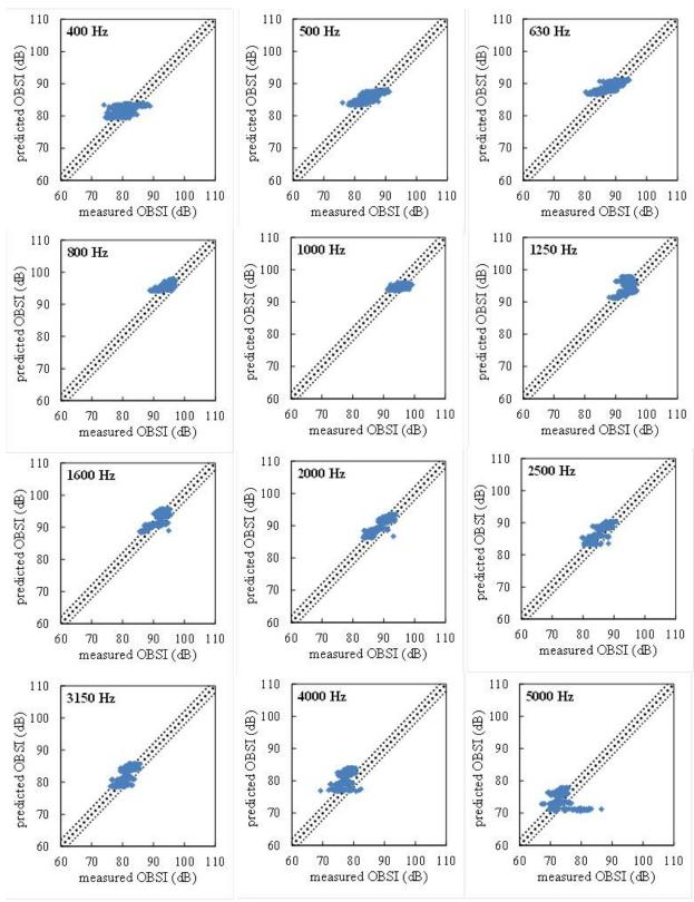
Figure 49. Measured and predicted one-third octave band levels, trailing edge, CTM model.
