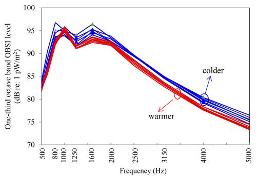
Figure 7: Variation in OBSI spectra with pavement temperature for cell 19. Blue lines correspond to colder temperatures (near 0°C); red lines correspond to warmer temperatures (near 10°C).
