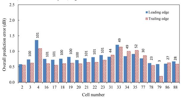
Figure 39: RoboTex Model accuracy by cell. Numbers above the bars indicate the number of OBSI measurements included for that cell in the model.
