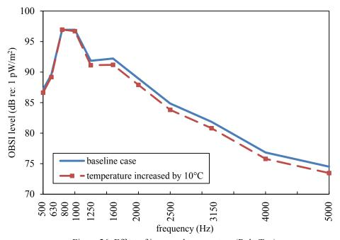
Figure 26: Effect of increased temperature (RoboTex).
