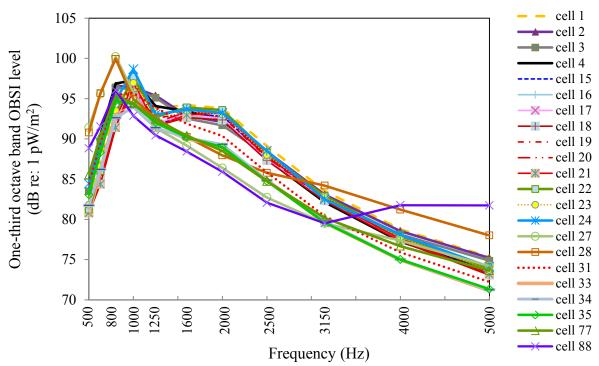
Figure 11: OBSI spectra for 22 pavements included in one-parameter texture model.
