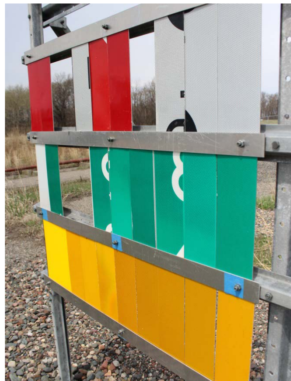
Researchers will use a test deck to study retroreflectivity and color readings to determine the life of sign sheeting material.
