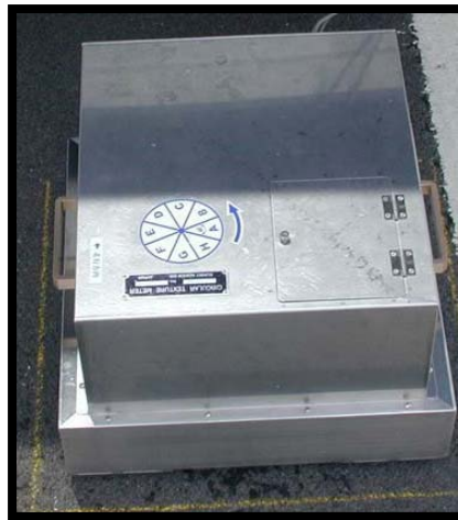
Figure 4: Circular Texture Meter
