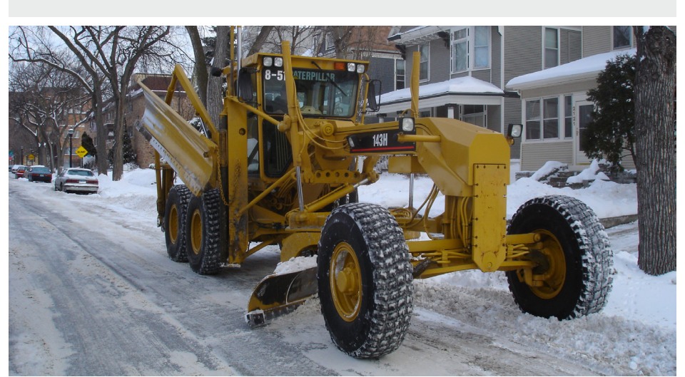
Motor Grader with wing plow attachment (currently in the raised position)
