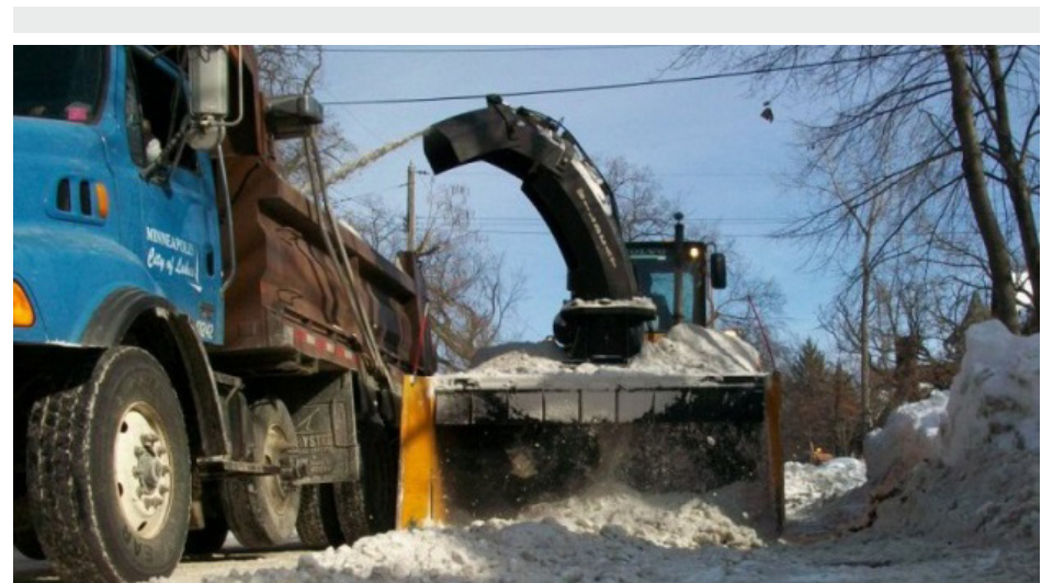
Snow removal using trucks and loader with blower
