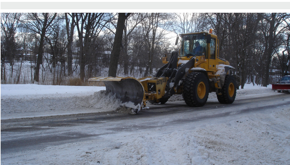
Loader with reversible front plow, which allows snow to be thrown to the left and right, as needed
