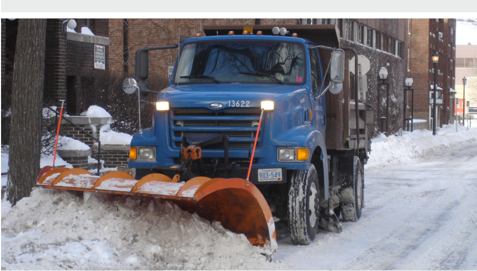
Dump Truck with underbody and front plows as well as a material spreader
