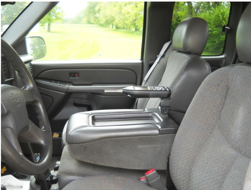
Figure 4.7 Location of Sound Level Meter in the Pickup
