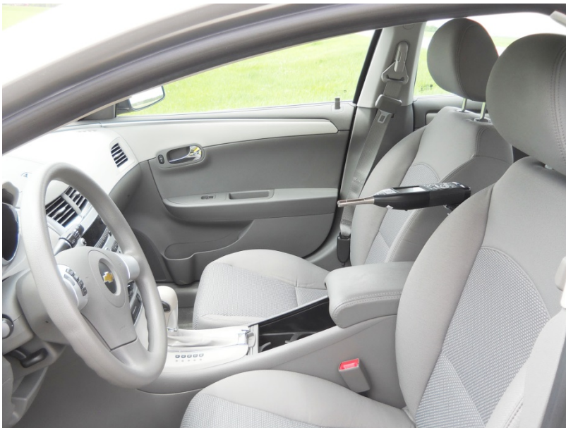
Figure 4.5 Location of Sound Level Meter in the Passenger Car
