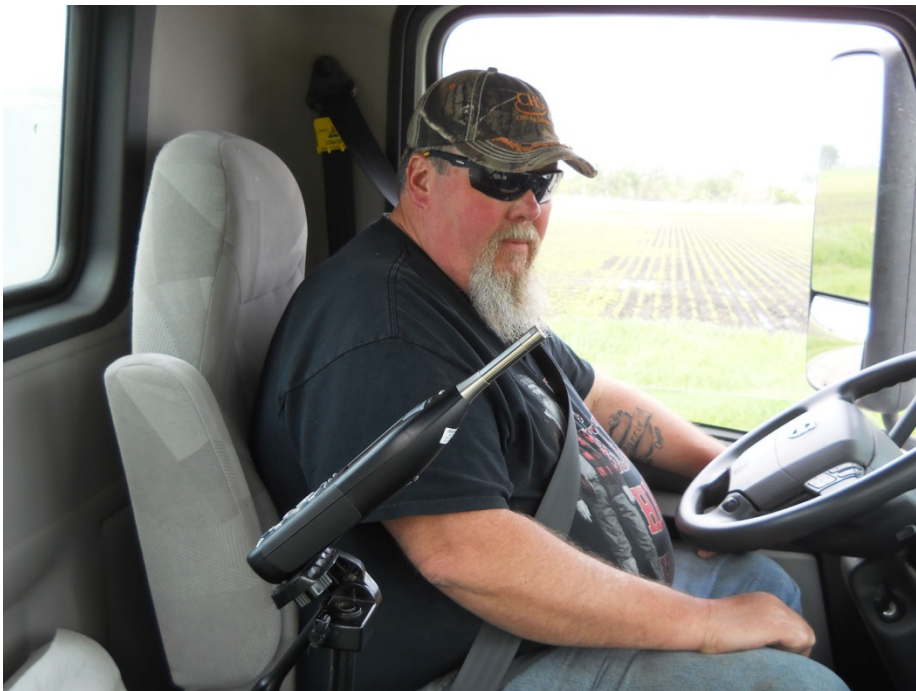
Figure 4.9 Location of Sound Level Meter in the Truck Cab
